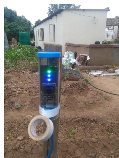
Above Left: The soil auger used for gravimetric soil water sampling and for drilling the holes for the Chameleon water sensors. Above centre: Sylvester installing a Chameleon sensor in a trench inside a tunnel. And Above right: The automatic reader for water availability attached to the Chameleon sensor in a trench bed. These are uploaded via the internet using cell phones on a weekly basis.
