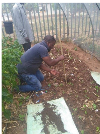
Above Left: The soil auger used for gravimetric soil water sampling and for drilling the holes for the Chameleon water sensors. Above centre: Sylvester installing a Chameleon sensor in a trench inside a tunnel. And Above right: The automatic reader for water availability attached to the Chameleon sensor in a trench bed. These are uploaded via the internet using cell phones on a weekly basis.
