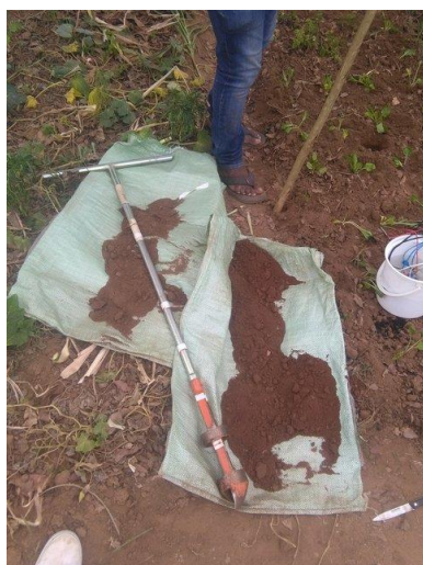
Above Left: The soil auger used for gravimetric soil water sampling and for drilling the holes for the Chameleon water sensors. Above centre: Sylvester installing a Chameleon sensor in a trench inside a tunnel. And Above right: The automatic reader for water availability attached to the Chameleon sensor in a trench bed. These are uploaded via the internet using cell phones on a weekly basis.
