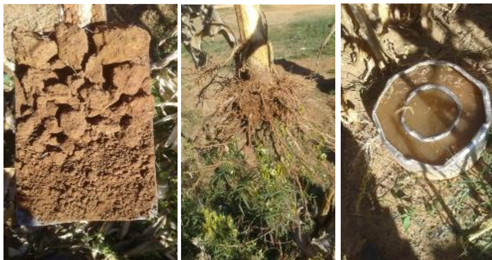
Figure 9: From Left to Right: A spade of her soil graded to show large clods but little structural integrity; An example of root size and depth of one of her maize plant - showing quite shallow rooting and the double ring infiltrometer set up for readings. The walls of the rings are quite battered due to extreme difficulty of getting the rings into the soil
