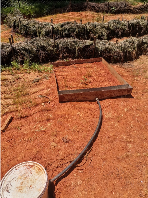
Figure 1: Run-off plots have been installed at different positions within the gully that is being restored through the demonstration funded through the WWF-PepsiCo upper uThukela Partnership.
