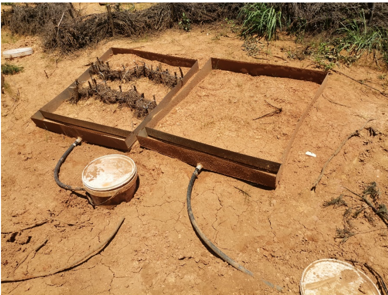
Figure 2: Mini brushpacks constructed in one run-off plot to allow for a comparison with the adjacent plot.
