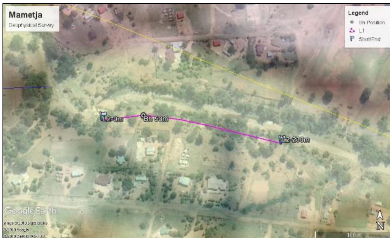
Above: Assessment of Line 2 for borehole options. This line is close to the river in Sedawa and thus also has the greatest possibility of finding a strong source without deep drilling
