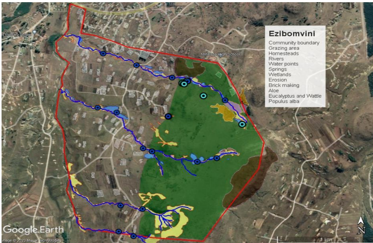
Figure 3: The Ezibomvini map with features of the middle stream shown in the white block within the picture. This includes water points, small wetlands, brickmaking activities and erosion along this water course. The light blue pattern shows the wetland patches along this stream. The yellow indicates erosion and the dark brown/purple patches within the block brick making areas.
