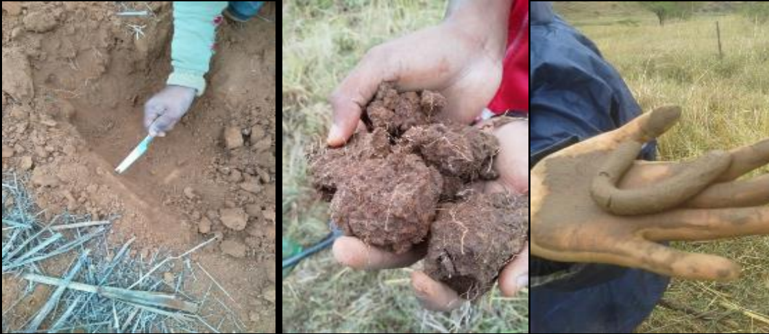
Above Left-Right: Doing the bulk density test using a knife blade. A clod of earth showing good aggregation, organic matter and fine root system. A soil sausage showing the high clay content of the soil.
