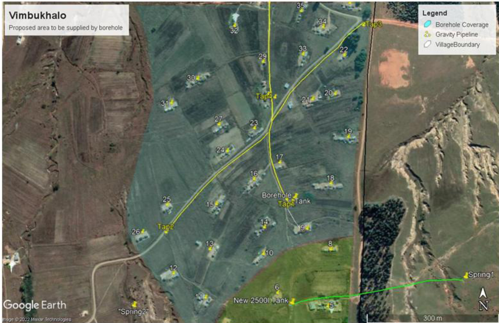
Fig 20: Example layout of borehole supply to village standpipes(map 1 of 2)
