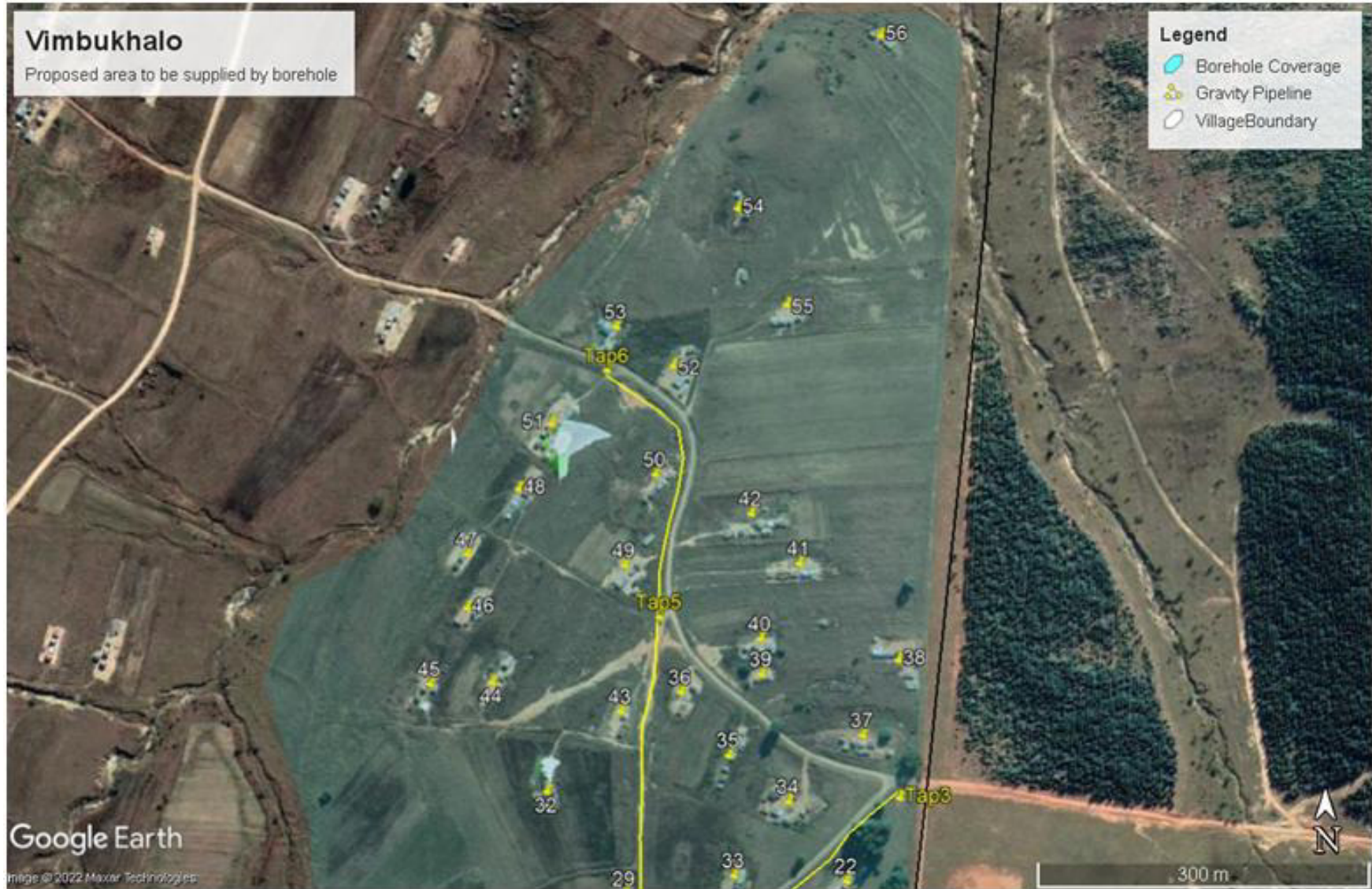
Fig 21: Example layout of borehole supply to village standpipes (map 2 of 2)
