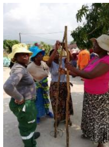
Figure 32: Right: One of the sub groups of participants busy constructing their line level
